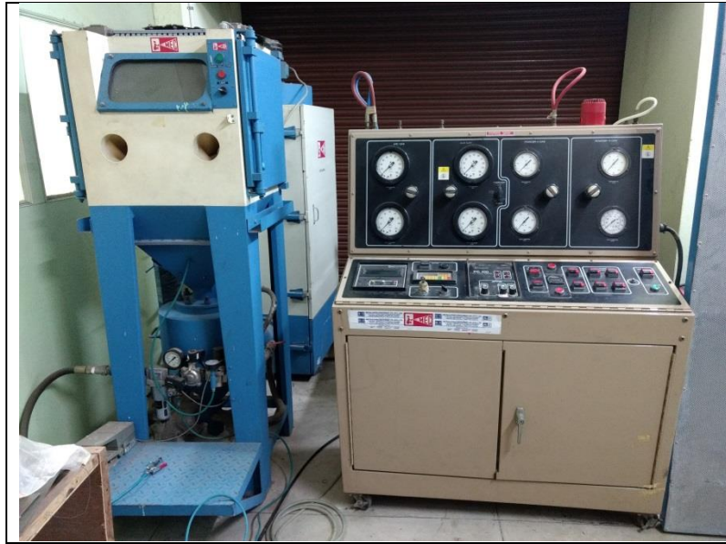
Sand Blasting Unit developed under the project sponsored by Department of Science and Technology, N. Delhi and installed in the thermal spraying laboratory
