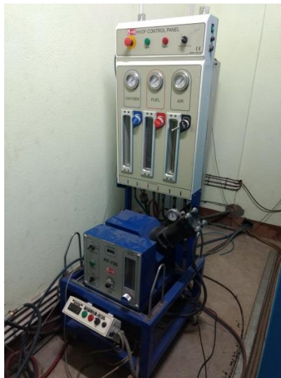
High velocity oxyfuel coating unit (Model No.: Hypojet – 2700, Made: MEC, Jodhpur) developed under the project (as a PI) sponsored by Naval Research Board and installed in the thermal spraying laboratory.
