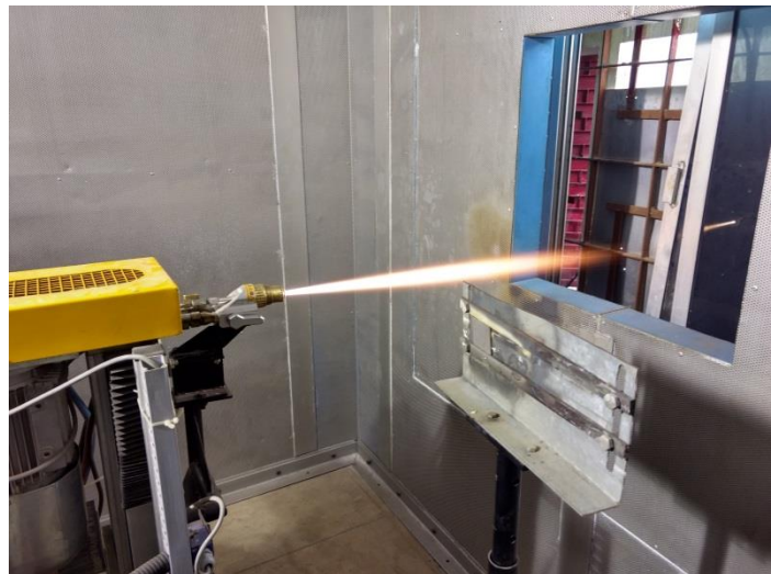
High velocity oxyfuel coating unit (Model No.: Hypojet – 2700, Made: MEC, Jodhpur) developed under the project (as a PI) sponsored by Naval Research Board and installed in the thermal spraying laboratory.
