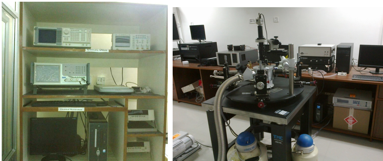
Figure 4 left panel shows I – V, and impedance spectroscopy measurement facilities. Right panel shows probe station for the measurement of dielectric and ferroelectric characteristics of thin films
