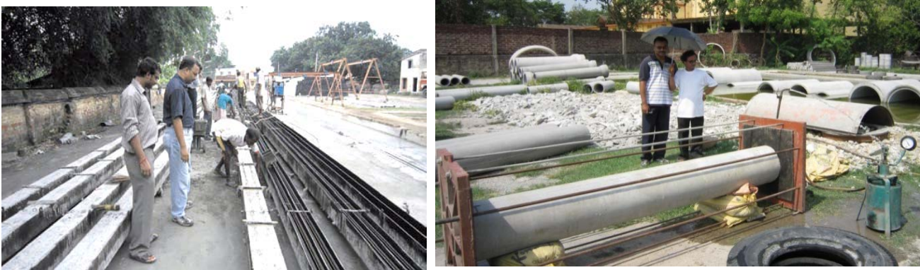
Figure 2 Left: Inspecting the fabrication of jute fiber reinforced pre-stressed electric pole. Right: Prof. Majumder inspecting the water leak testing of fabricated jute fiber reinforced sewer pipes
