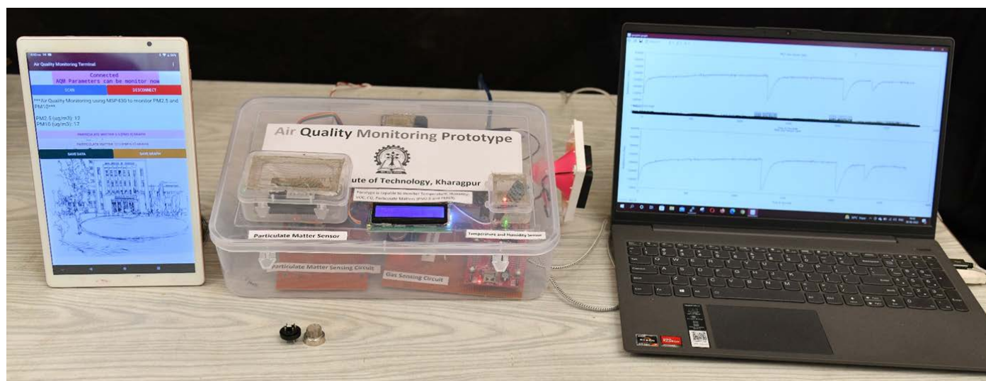
Figure 3 The developed AQM system connected with a laptop to display response transient during gas sensing and with a Tab (through blue tooth) for PM sensing. The LCD screen displays the temperature and ambient humidity. The developed Taguchi type sensing elements are shown separately.
