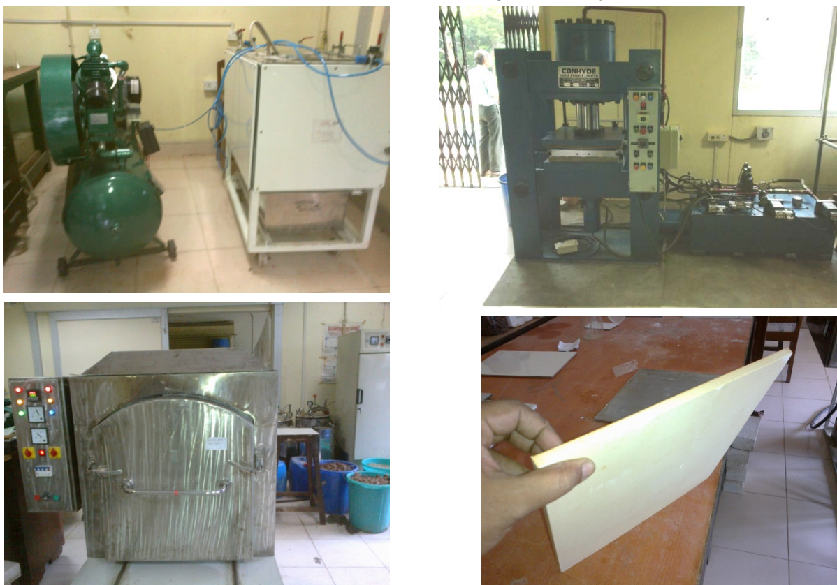
Figure 6 Clockwise from top: Fluidized bed mixer, 160 MT hydraulic press, furnace and biscuit fired fly-ash tile.
