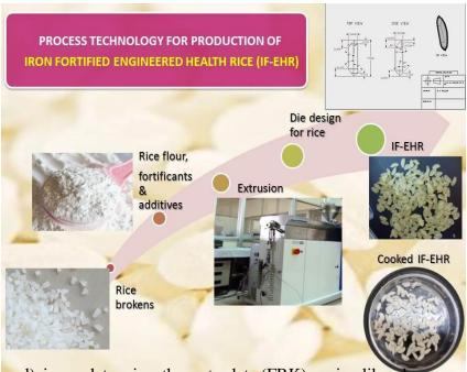
a rice shaped die (specially designed) is used to give the extrudate (FRK) a rice-like shape.
